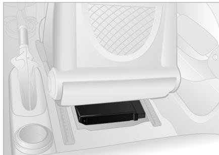
Map CDs/DVDs are inserted in the navigation computer. It is located in the floor beneath the right seat and is protected by a cover.
